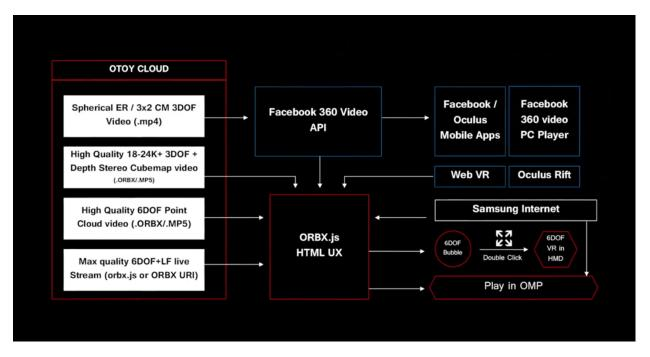
At the core of a serialized ORBX file is a simple virtual disk system and a single high level XML index file representing a root render graph to be evaluated, with optional inputs (camera view projection and position for example) and at least one output (usually a render target buffer with two or more dimensions).
