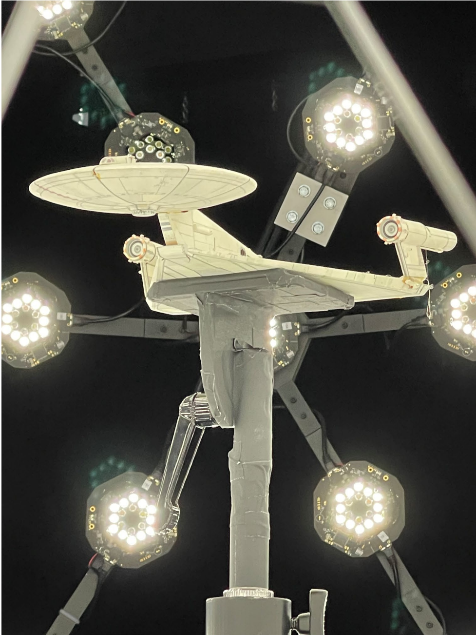
Scanning Star Trek "Planet of the Titans" physical model in OTOY's LightStage
